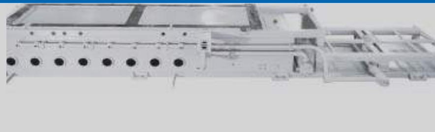
High rigidity injection unit base
